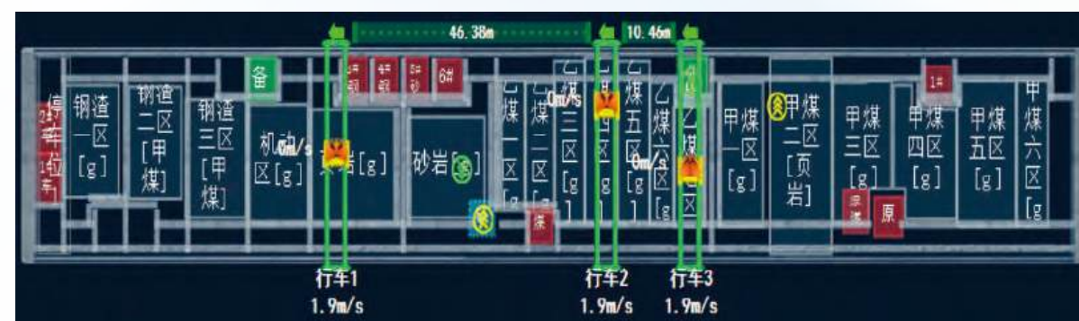
Multi-crane Collaborative Operation
